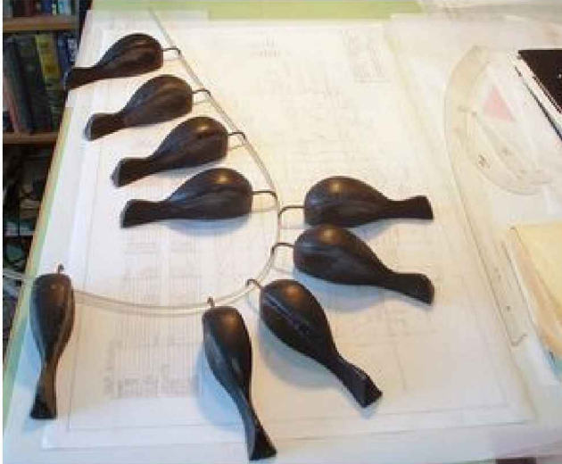
Figure 4-11. Splines were originally created using bendable wood and “ducks,” and were used as a draftsman tool to fit curves. Photo courtesy Bob Perry.
